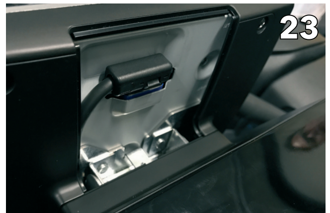
Insert the connector into the screen
