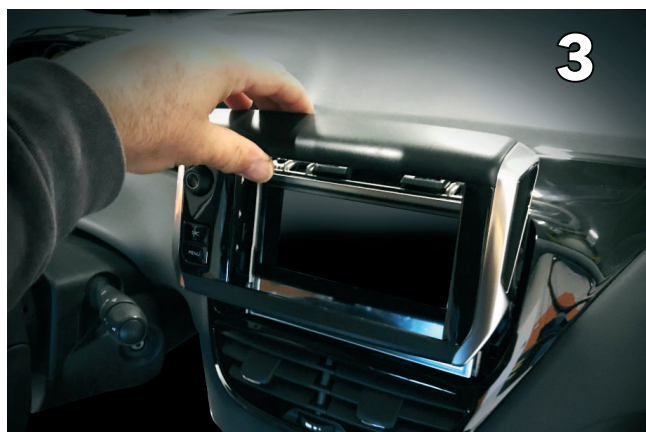
Pull upwards to remove and disconnect buttons
