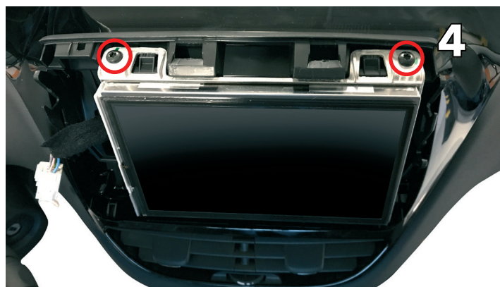
Remove two Torx screws on top
