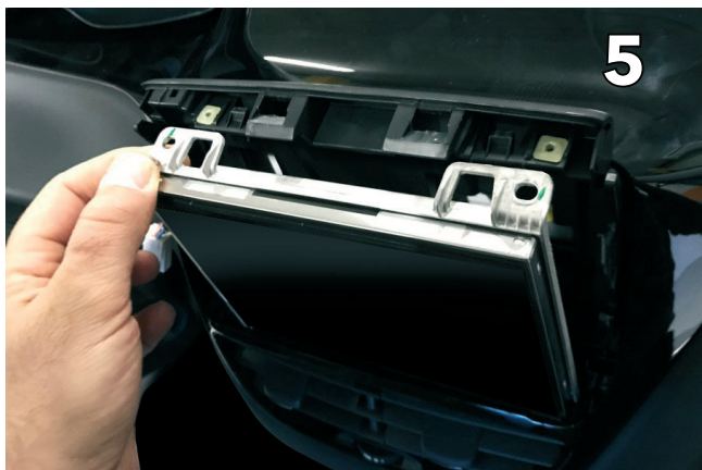
Remove the screen by pulling it towards you
