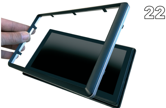
Install the front cover and chrome trim bezel on the screen
