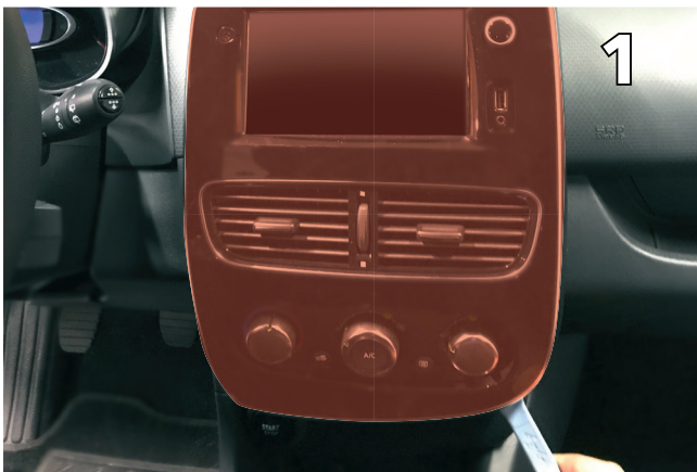
Remove the front panel using a trim tool
