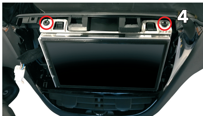
Remove two Torx screws on top
