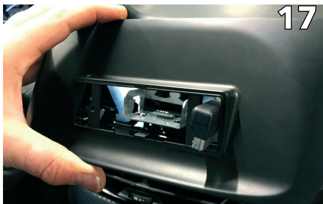
Install the dashboard cover (Make sure to put the display through)
