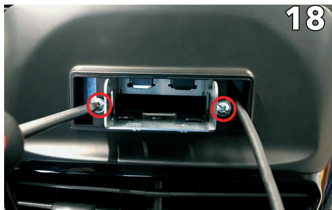
Secure the dashboard cover with the supplied screws
