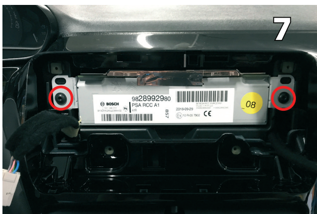
Remove the original stereo
