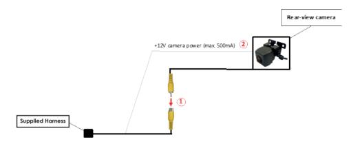
Connect the video RCA of the rear-view camera to the female RCA connector of the supplied harness.
