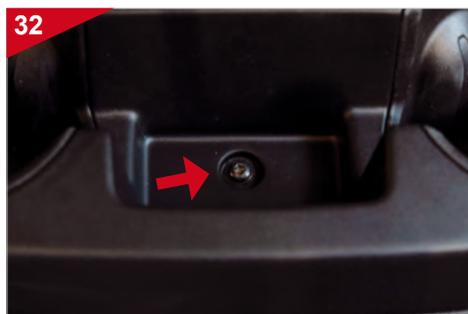
Remove the screw under the rubber insert.
