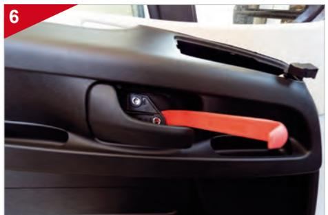
Lever out the door handle with a mounting wedge.
