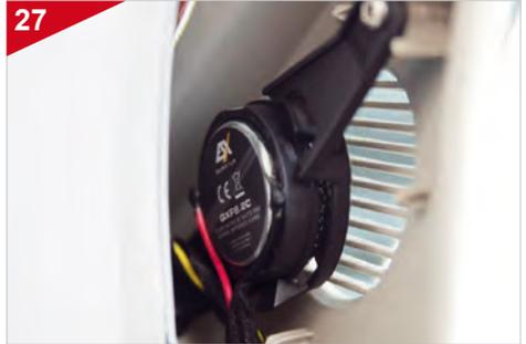
Replace the original tweeter with the ESX tweeter. Use the original tweeter bracket for this.
