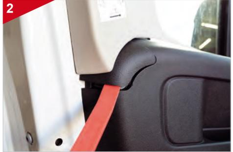
First, the door panel must be removed. To do this, loosen the cover on the bottom left of the window with a mounting wedge.
