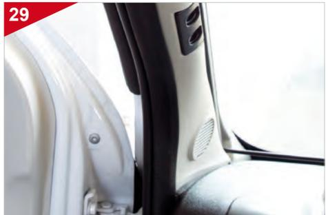
Fold the cover back to its original position and reinsert the rubber seal into the door opening.
