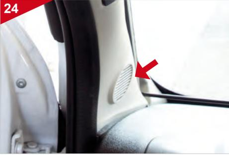
Start installing the tweeters on the driver's side. Then repeat all installation steps on the passenger side.
