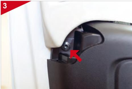
Remove the screw at the bottom left of the window.
