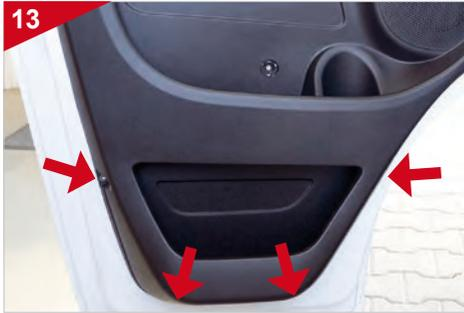
Remove the remaining four screws on the door panel as marked above.
