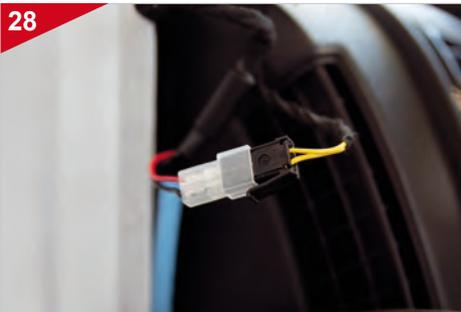
Connect the ESX tweeter to the vehicle's connector plug.
