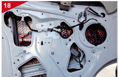
**OPTIONAL:** To do this, remove the white foam and glue the aluminum butyl panels inside the door.
