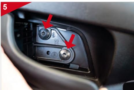
Remove the two screws behind the door handle.
