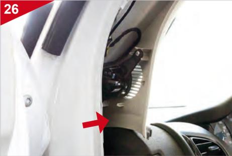
Then carefully fold out the cover of the tweeter. Then unplug the connector from the original tweeter.
