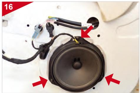
Disconnect the connector at the top of the speaker, and then remove the three screws on the speaker.
