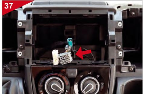
Plug the two ISO plugs into the corresponding ISO sockets (B and D) on the amplifier wiring harnesses supplied.
