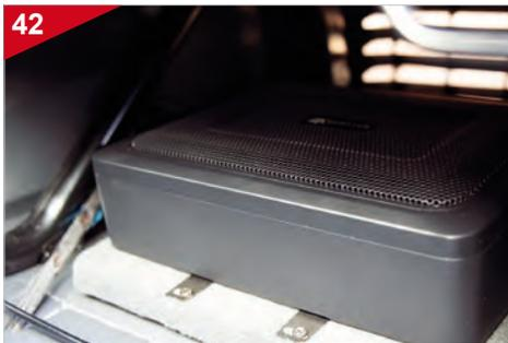
**OPTIONAL:** For example, an active subwoofer system like the ESX Q168A can be mounted under the driver's seat.
