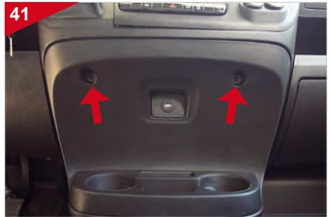
After you have made the settings on the amplifier (see page 23) and performed a successful function test, reattach the cover on the lower center console.
