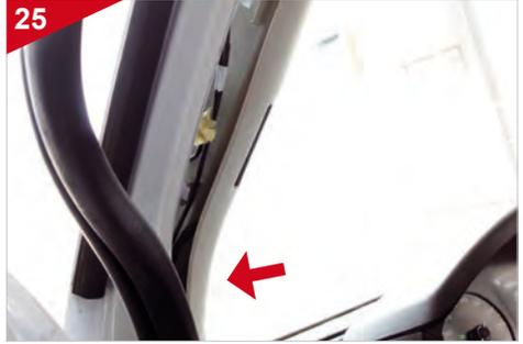
Lever out the rubber seal of the door opening with a mounting wedge and carefully pull it out at the appropriate point.
