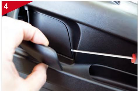
Remove the cover behind the door handle using a suitable screwdriver.
