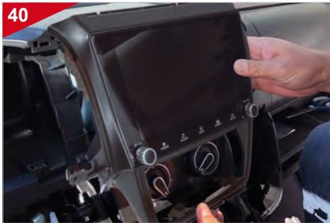
Reinstall the original radio or naviceiver in the dashboard.
