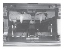
5 In order to clear space for the radio, cut and remove the plastic parts along the lines highlighted in the picture.
