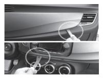
3 Remove the original facia by leveraging as shown in the picture.
