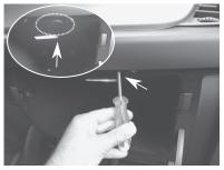
2 Remove the circular lid in the glove compartment and unscrew the retaining screw.
