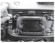
4 Unscrew the four screws and remove the original head unit; disconnect the plugs.
