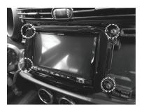
8 Connect all cables, verify the proper functioning of the system and insert the unit into the housing. Place the facia plate supplied and screw the four screws as shown in the picture.
