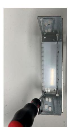
a) Fix plastic cover to bracket holder using the 4 screws supplied in the kit.
