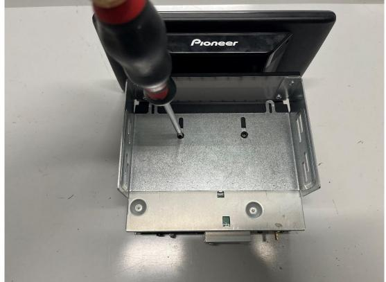
**b)** Attach the previously pre-assembled bracket holder + cover to the silver box of the radio with the **2 black** screws supplied in the kit.
