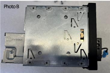
2) Insert the aftermarket cage (photo A) and fit the supplied 2Din bezel (photo B).
