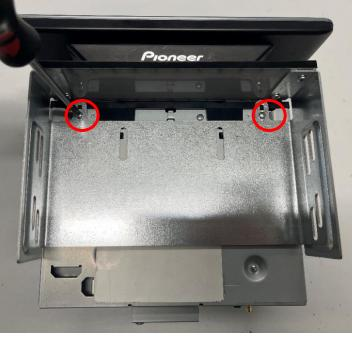
c) Fasten the previously pre-assembled bracket + cover to the silver box of the radio with the 2 silver screws and the 2 thicknesses supplied in the kit.
