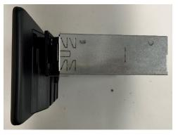
5) Slide the unit into the metal cage until it's locked, then lock the plastic frame.
