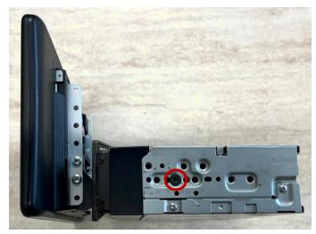
3) Use the **black screw** to create a shim (1 on each side as shown), so that the spring brackets do not sag. **ATTENTION:** Perform this procedure only for compatibility with SPH-EVO950DAB.
