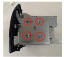
6 Fix the facia plate to the radio by tightening the 8 screws (4 per side) supplied in the Radio Kit
