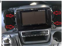
7 Connect all cables and verify their functions, tighten the 4 screws saved in the step n°2 as indicated in the picture.
