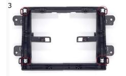
3 Remove and save the 4 clips circled found to the back side of the OEM facia plate.
