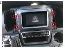
2 Remove the OEM Air Vents. Remove and save the 4 screws circled in Red.
